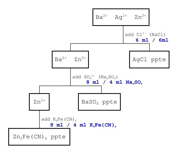
The presence of a precipitate (ppte) is takes as proof of the presence of the cation in the mixture. Removal of the precipitate is accomplished with the centrifuge.
