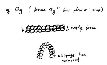
when stressed, metal ions can slip past each other without interrupting the metallic bond (note that the electrons remain in constant wandering motion the whole time)
