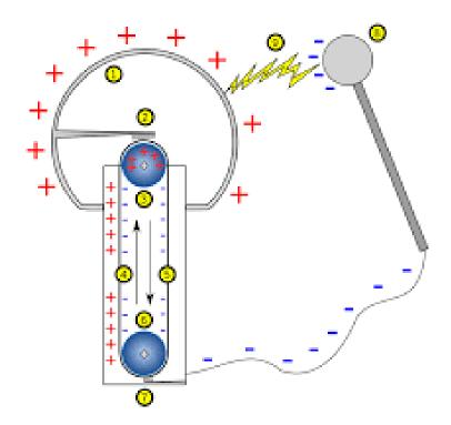
At the top pulley the rubber belt picks up electrons and then drops them off at the bottom pulley. The lack of electrons at the top pulley creates a positive charge. Since the aluminum sphere is a conductor, the positive charge will spreads out evenly over the sphere. Objects in contact with the sphere become positively charged. When the postive charge becomes large enough, a sudden static discharge or spark occurs to neutralize the Van de Graaf generator.
